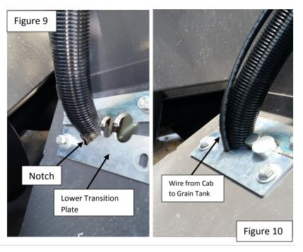
that wire in grain tank is comfortable. Finish reinstalling lower transition plate with blanks and bolts.
